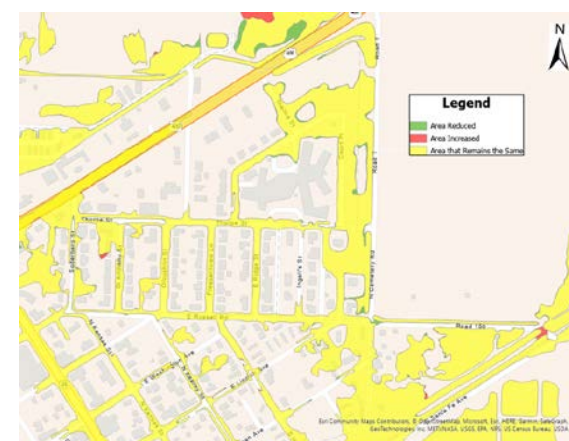
Alternative 2 – adding detention basins west of KS-25 and northwest of the intersection of US-50 and Road T.
