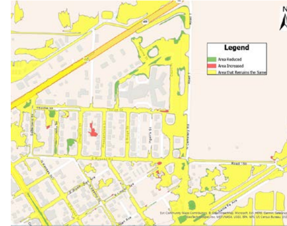
Alternative 3 – adding inlets near the intersections of Harolds Place and Court Place and Thorpe Street and Court Place.
