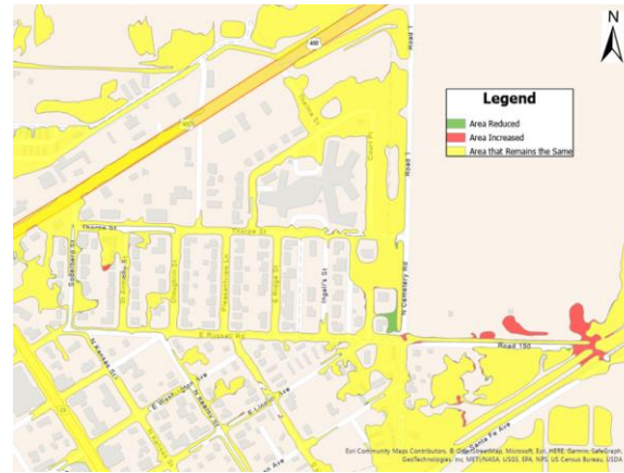
Alternative 1 – modification of the existing culvert S10, located north of the intersection of Russel Road and North Cemetery Road.
