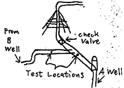
Flow test under "normal" conditions:
