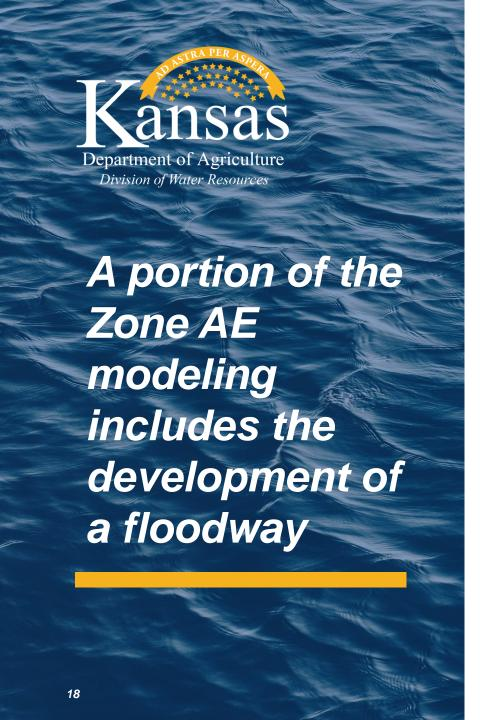
A Floodway is the area within the floodplain that must be reserved in order to discharge the base flood without cumulatively increasing the WSE by more than 1.0 foot.
