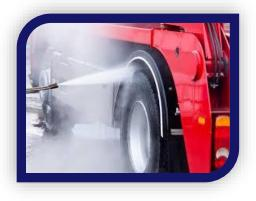
debris as possible. Brush or scrape debris from the vehicle. Washing of the vehicle should follow. High pressure spraying equipment (i.e., 200 - 1000 psi) may help to clean wood pores, cracks and crevices. Clean the vehicle from top to bottom and wash the underside of fender wells and the vehicle frame. Apply an appropriate disinfectant with a low-pressure sprayer and allow its proper contact time to elapse. Also, clean and disinfect the interior of the vehicle prior to leaving the premises.
