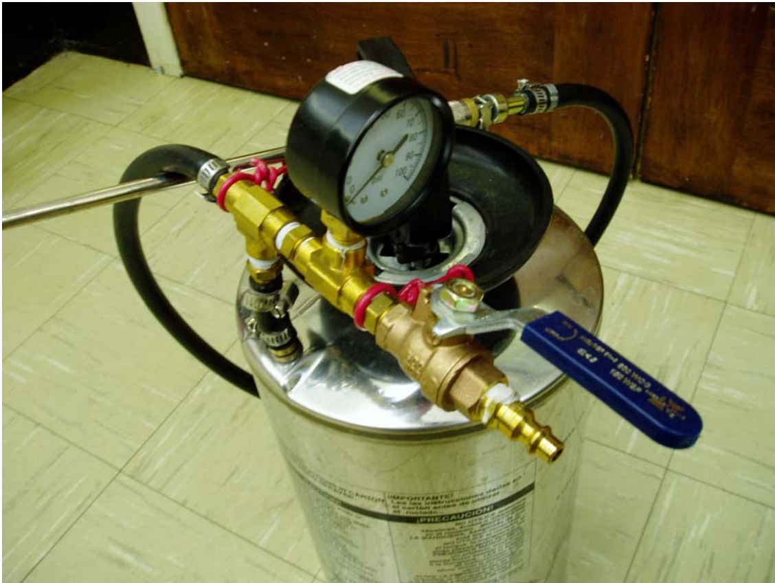
Figure 9. Close-up view of retrofitted garden sprayer
