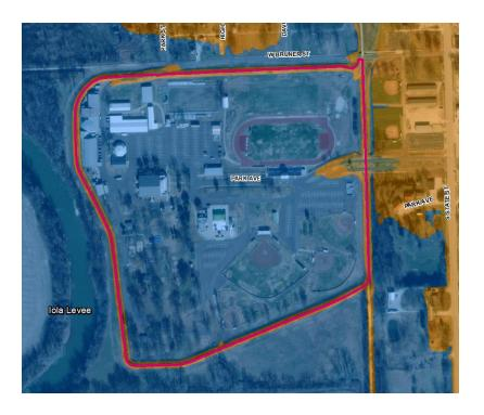
The new mapping is based on a Natural Valley Procedure which reflects the levee geometry in the hydraulic model but allows water to flow on either side of the levee.
