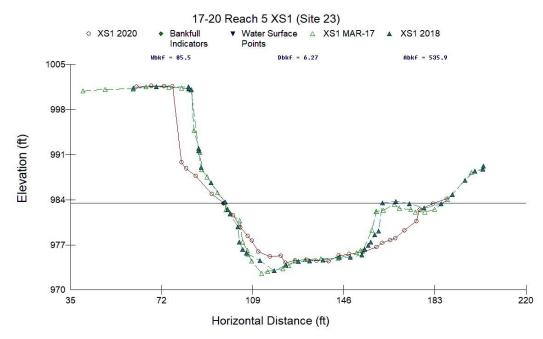
Figure C.1. Reach 5 Cross Section (XS) 1 at Site 23 Survey, March 2017, March 2018, and September 2020. This cross section went through the middle of woody revetment 1 (of 3) that was washed out by 2020.
