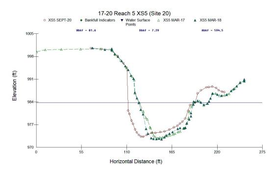
Figure C.5. Reach 5 XS5 at Site 20 Survey, March 2017, March 2018, and September 2020. This cross section is between revetments 5 and 6 (of 7) that was washed out by 2020.
