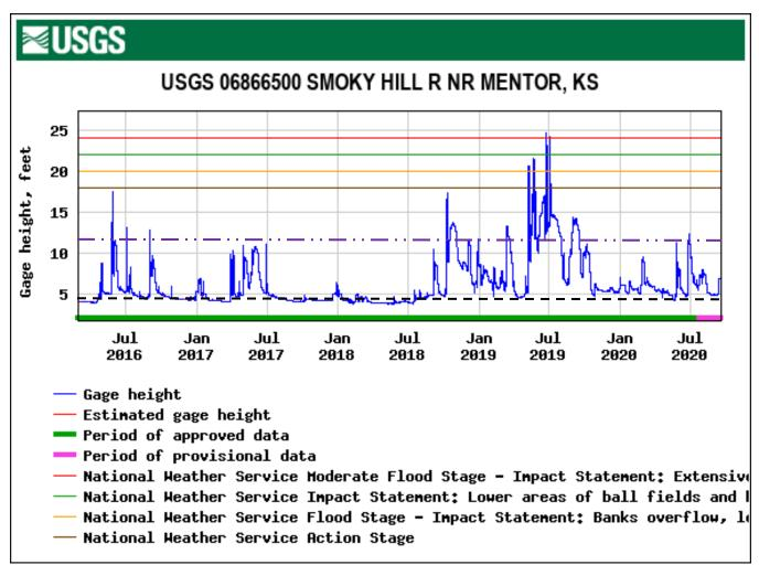
Figure 4. March 2016 through September 2020 Smoky Hill Flow Events recorded at USGS Gage near Mentor, KS (#06866500). The purple dashed line represents the bankfull stage, the black dashed line represents the stage of safe data collection.
