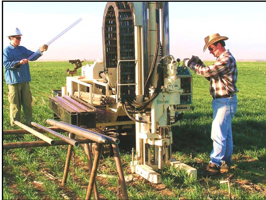
Figure 63. Geoprobe Sampling of Soils to 25 feet in the Spring of 2006.
