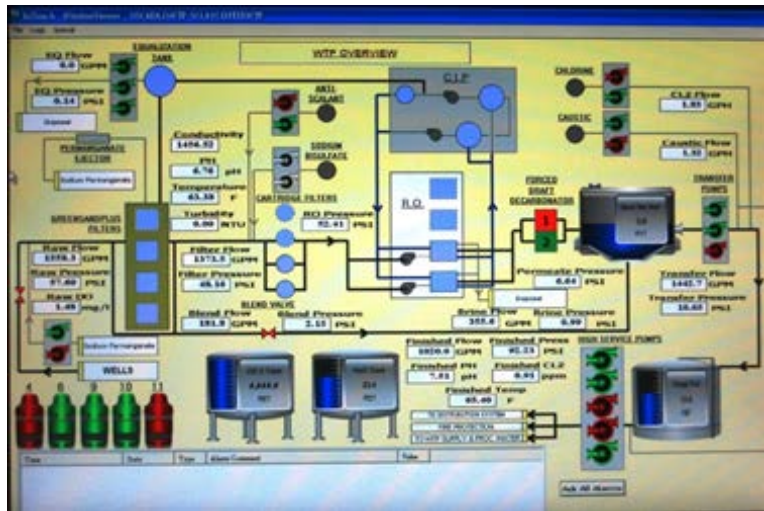
Photo 4 – Example SCADA screen interface
