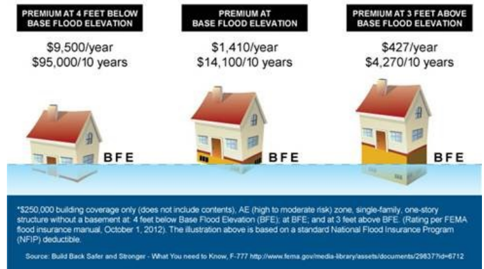
Above: Potential insurance premium savings from “freeboard,” or additional height above Base Flood Elevation (courtesy FEMA).
