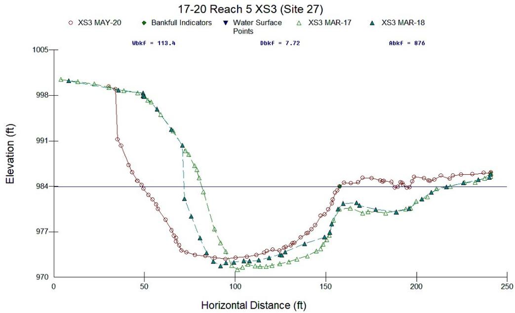
Figure C.8. Reach 6 XS3 at Site 27 Survey, March 2017, March 2018, and May 2020. This cross section is located just upstream of woody revetment 9 (of 9) that was washed out in 2017.
