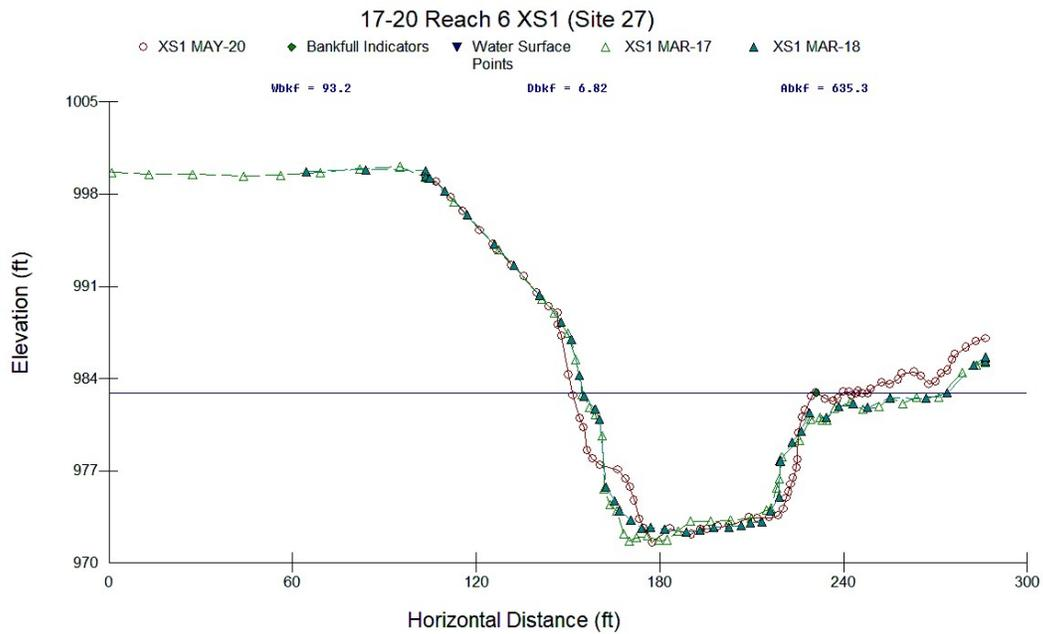
Figure C.7. Reach 6 XS1 at Site 27 Survey, March 2017, March 2018, and May 2020. This cross section is between woody revetment 1 and 2 (of 9) that still remains in 2020.
