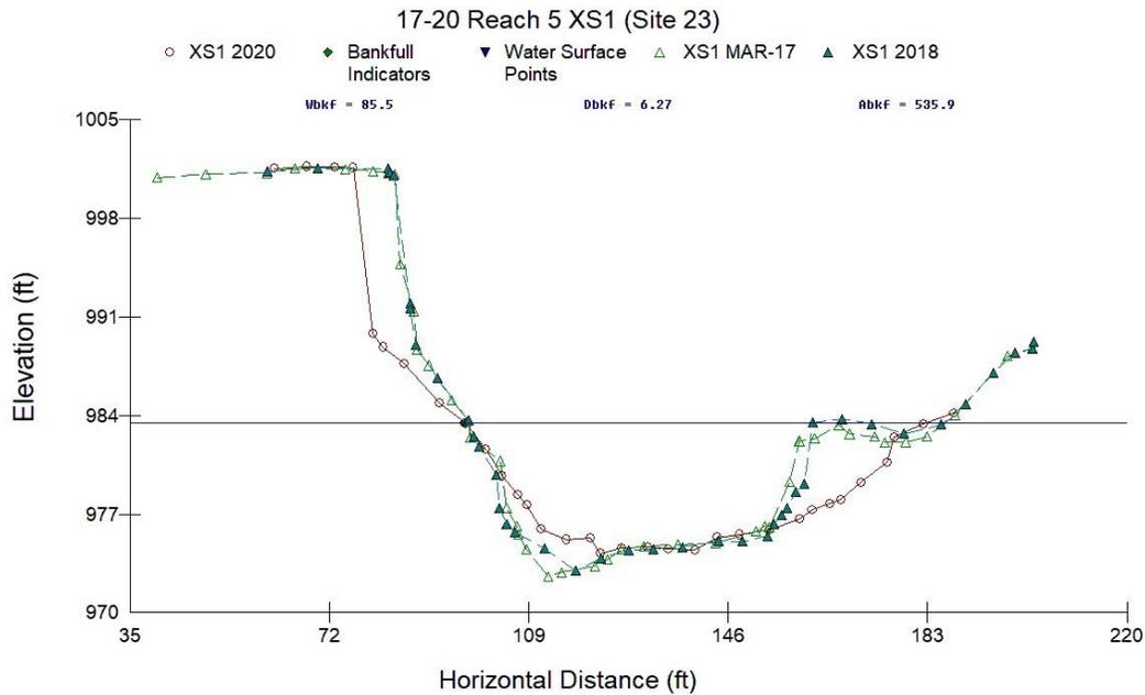
Figure C.1. Reach 5 Cross Section (XS) 1 at Site 23 Survey, March 2017, March 2018, and September 2020. This cross section went through the middle of woody revetment 1 (of 3) that was washed out by 2020.
