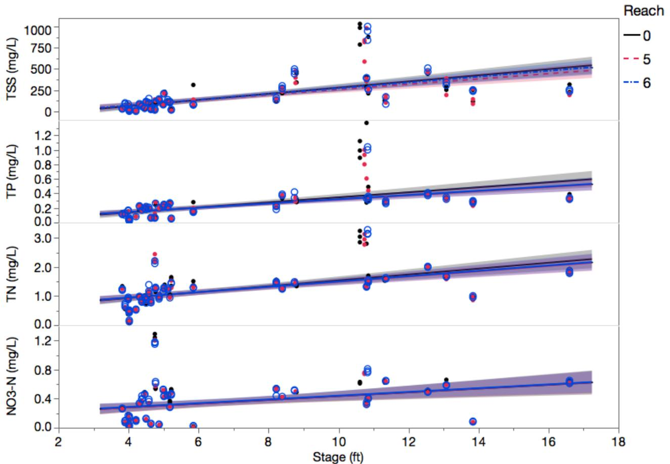
Figure 12. Relationship between Concentrations of Measured Water Quality Constituents and Stream Stage at the time of Sampling for Control (0), Reaches 5 and 6 (woody revetment treatments).
