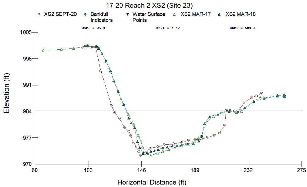
Figure C.2. Reach 5 XS2 at Site 23 Survey, March 2017, March 2018, and September 2020. This cross section went through the middle of woody revetment 3 (of 3) that was washed out by 2020.
