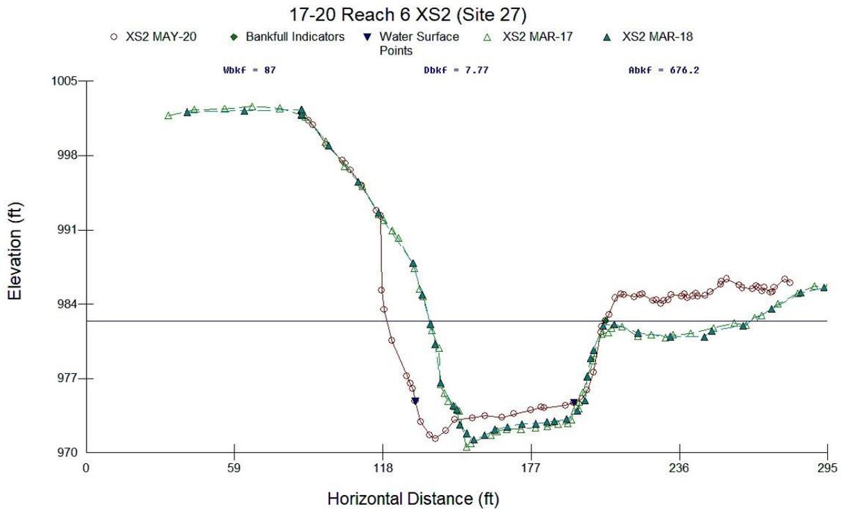
Figure 9. Example Cross Section (XS2) at Site 27 on Reach 6, March 2017, March 2018, and May 2020. This cross section went through the fifth (of 9) woody revetment and still remains in 2020.
