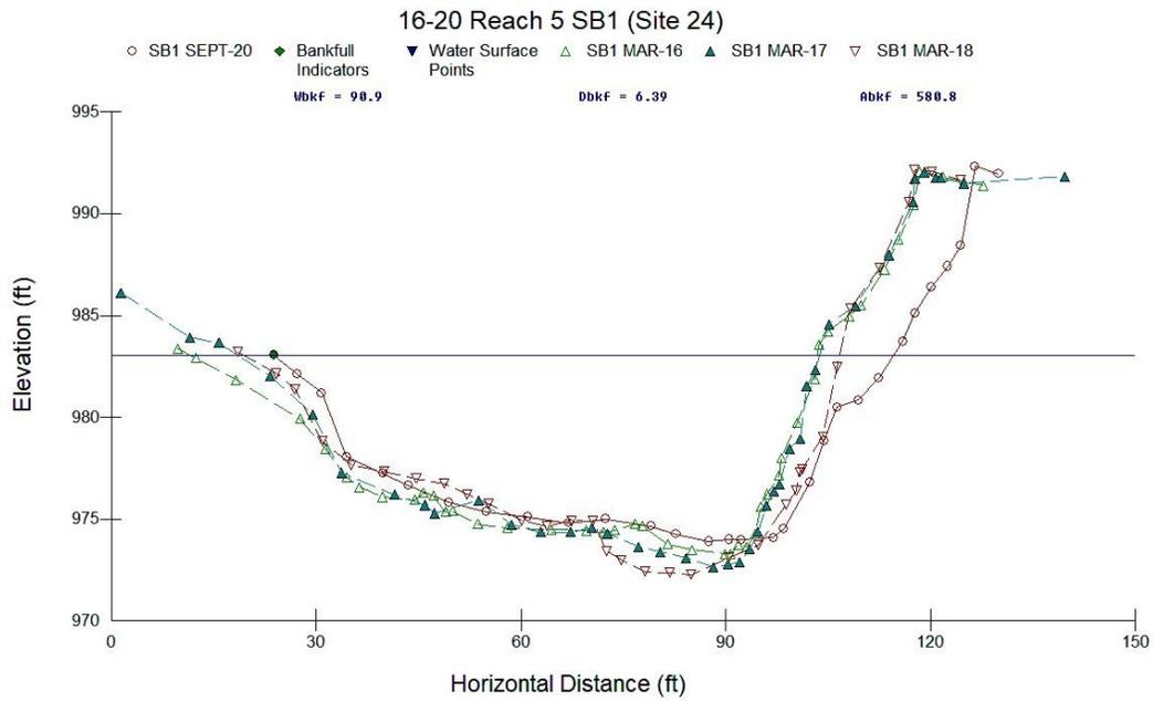
Figure C.6. Reach 5 Study Bank 1 (SB1) at Site 24 Survey, March 2016-2018, and September 2020.
