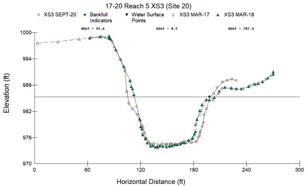
Figure C.3. Reach 5 XS3 at Site 20 Survey, March 2017, March 2018, and September 2020. This cross section is just downstream of revetment 1 (of 7) that still remains in 2020.
