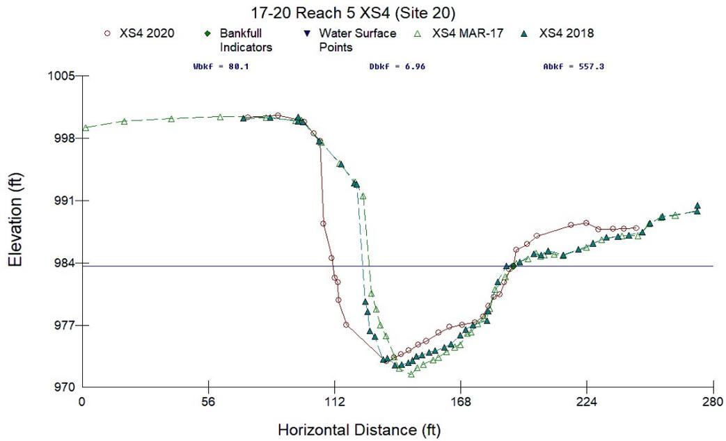
Figure C.4. Reach 5 XS4 at Site 20 Survey, March 2017, March 2018, and September 2020. This cross section is just downstream of revetment 4 (of 7) that was washed out by 2020.
