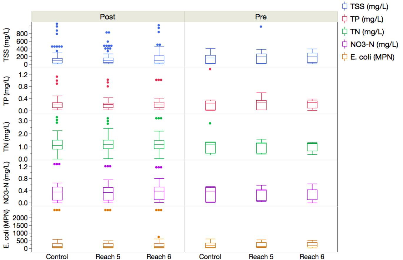
Figure 11. Box plots representing Distribution of Water Quality Data collected from Control (2) and Woody Revetment Treatment Reaches (5 and 6), Before (right panel) and After (left panel) Woody Revetment Installation. For reference, current TMDL or Water Quality Impairment Limits are: TSS = 50 mg/L; TP = 0.201 ppm; NO<sub>3</sub> = 10 mg/L.
