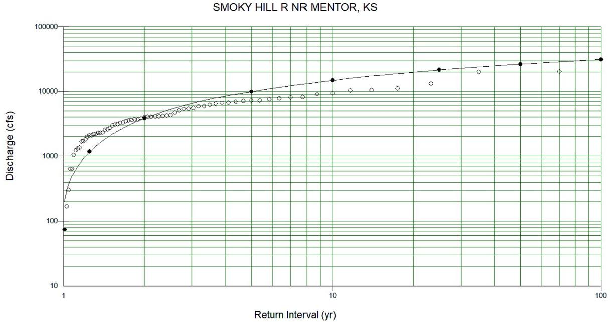
Figure A.1. Log Pearson Type III Flood Frequency Plot for USGS Gage #06866500 (1949 to Present)
