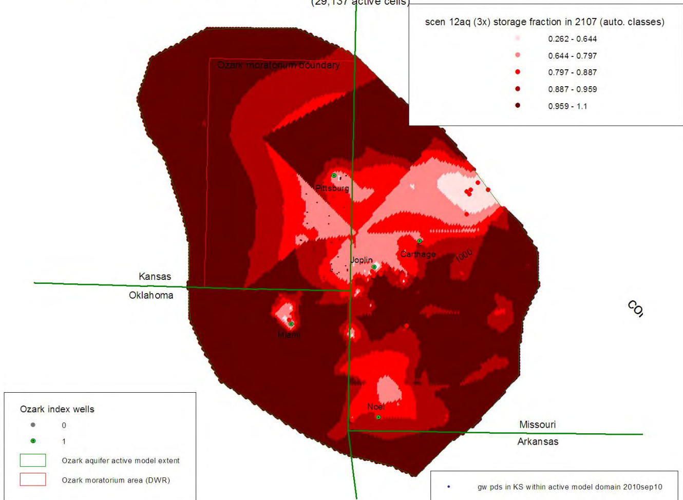
Fig. B6. Remaining storage fraction distribution at end of 2107, with automatically selected classes, for scenario 12aq (3x KS authorized quantity, 2x MO pumping), [scen12aq_remaining_storage_fraction_auto_classes.jpg]
