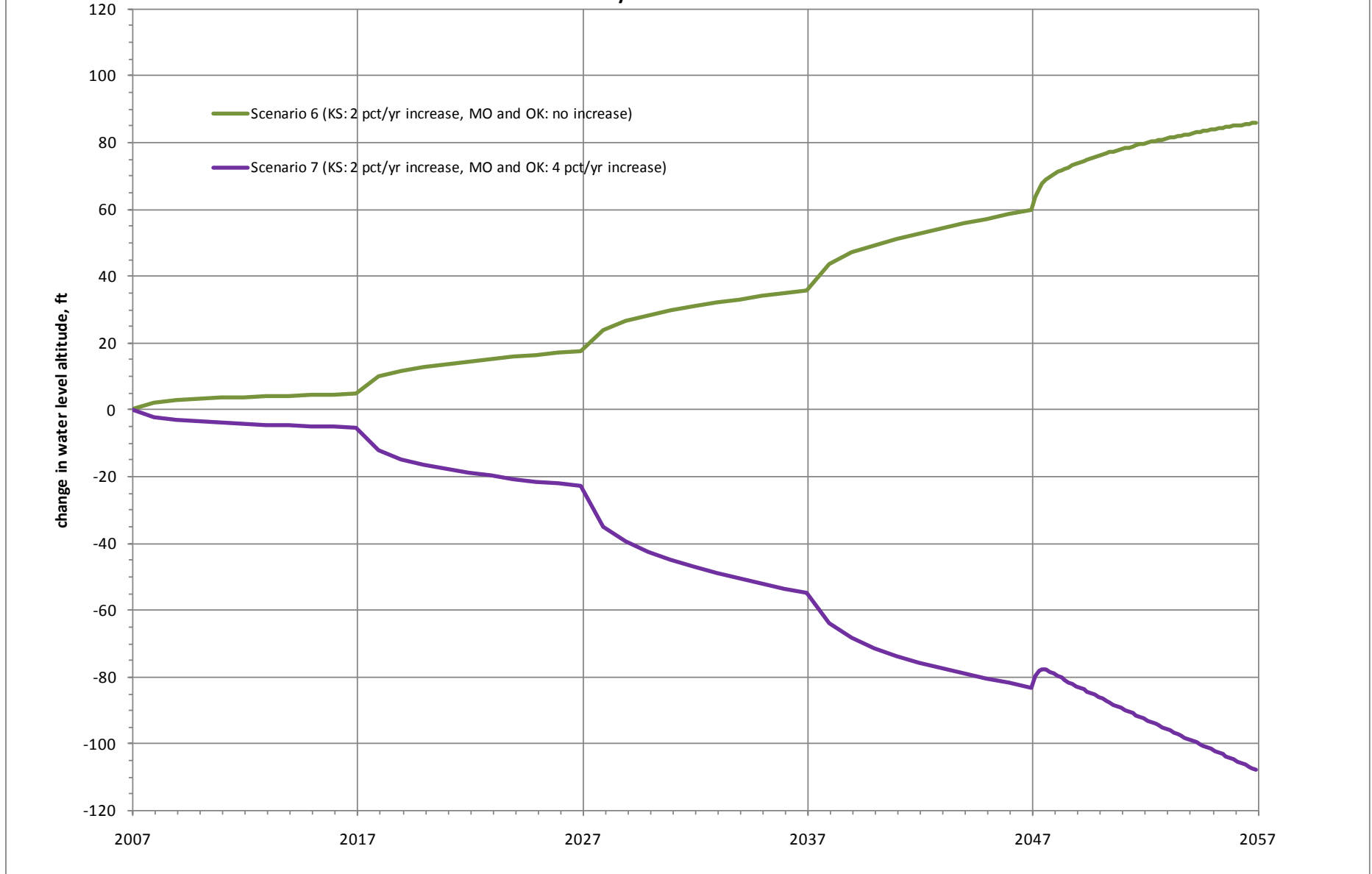
Fig. 12. Change in simulated water level with respect to Scenario 4 at node near Pittsburg, KS for years 2007-2057: Scenarios 6 and 7. Chart at aw2 in sheet Pittsburg_hydrographs in budget_baseline_alt_steps.xls.
